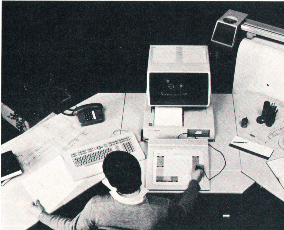
Fig. 1. The detached keyboard (Option G02) of the HP 9000 Model 520 Computer is available in Europe and complies with German ergonomic requirements specified by the ZH1/618 standard.
